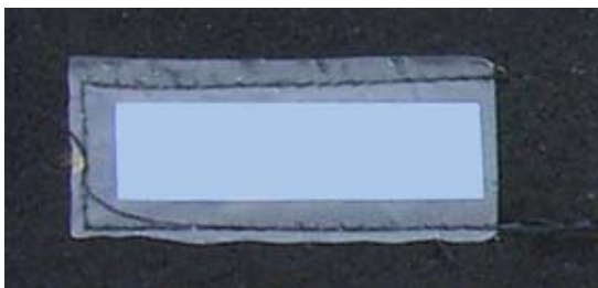
Hydrocarbon Detection Strip placed against outer layer.
