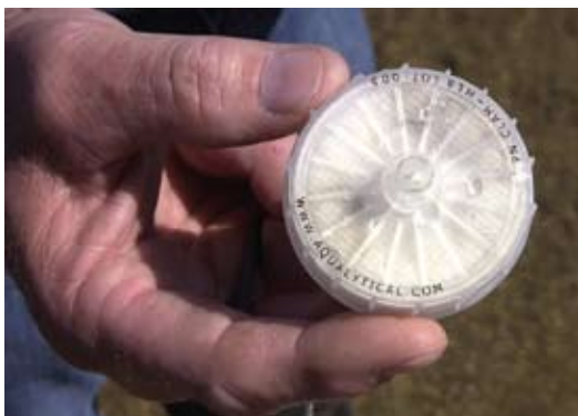
C.L.A.M. disk - that's all that gets sent to the lab.
